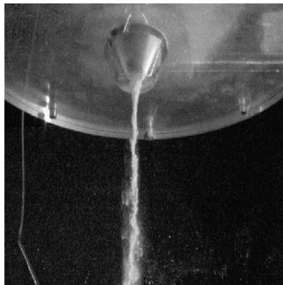
Fig. 3. Photo of the first 30 cm of a powder stream from the hopper outlet.
